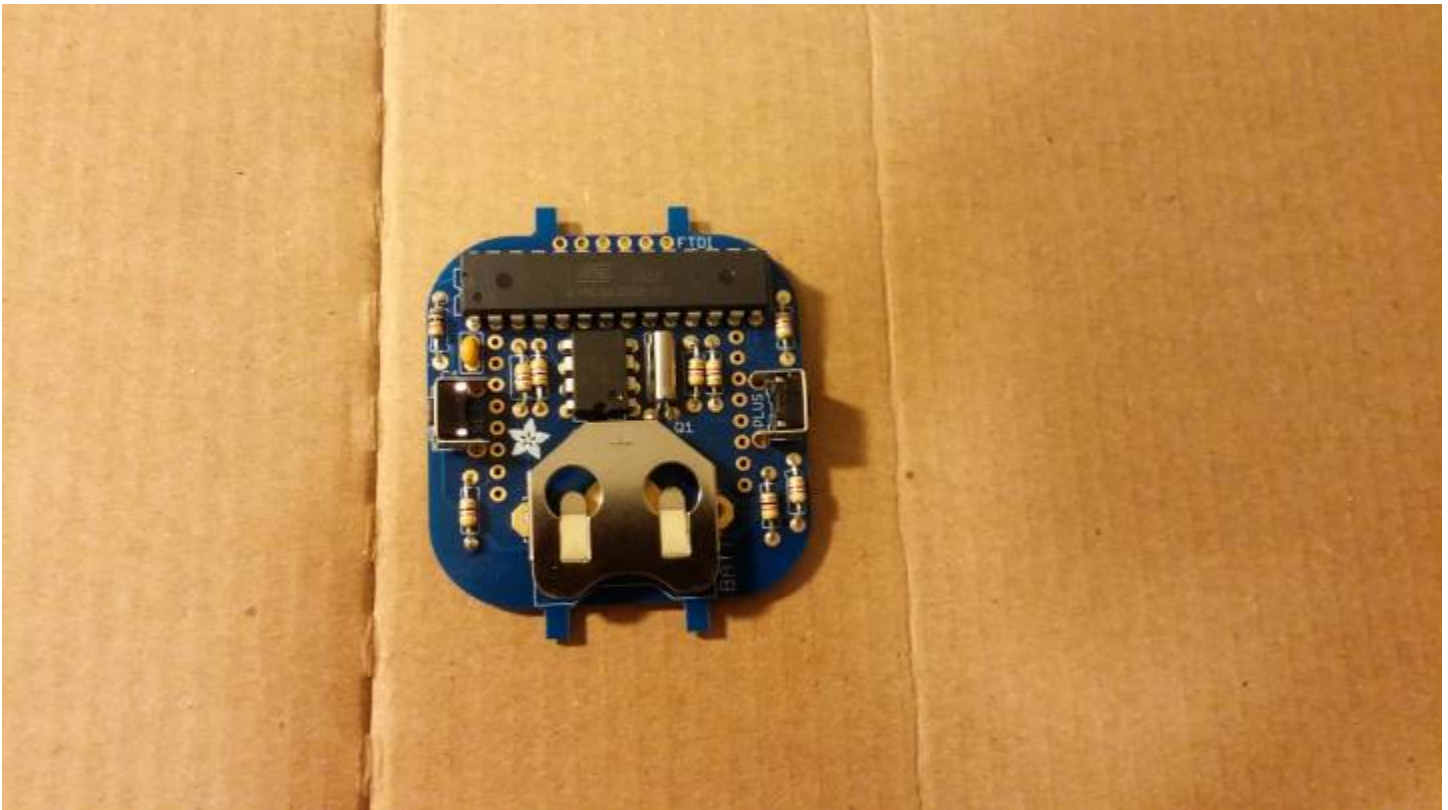
The battery holder, timing crystal, and buttons. It's getting pretty busy on the board!
