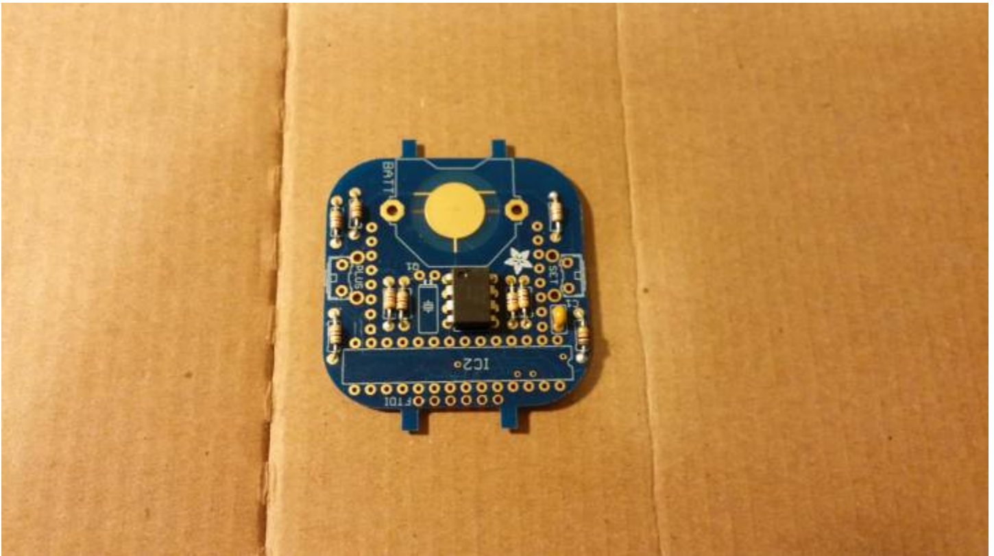
Our first chip – the DS1337. This one keeps track of the time for us.
